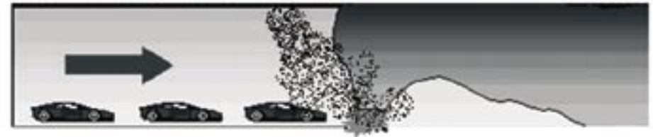
Figure 1 - Smoke displacement with longitudinal ventilation [11]
