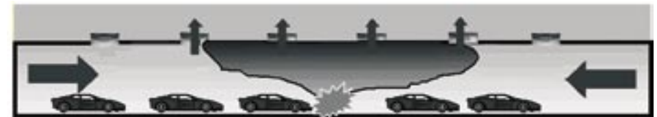
Figure 2 - Smoke stratification with transverse ventilation [11]
