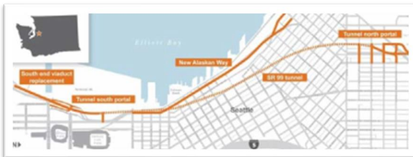
Figure 3 - SR 99 Tunnel alignment
