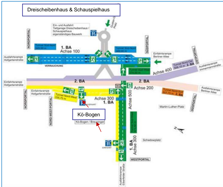
Figure 7 - Emergency exits – Overview
