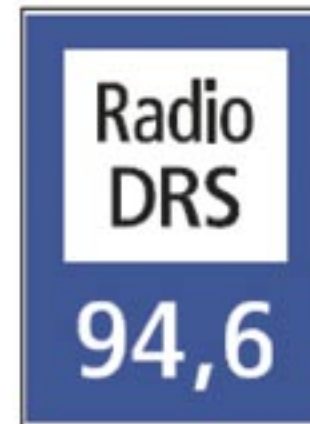
Figure 19: Sign F14 of the Vienna Convention to indicate the frequency that can be received in the tunnel
