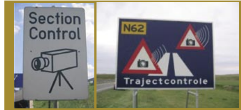
Figure 17: Examples of signs to warn drivers that there is section (TRAJECTORY) control
