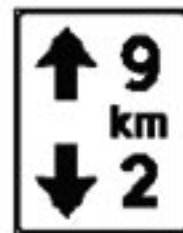
Figure 27: Norwegian example of indication of the remaining length of tunnel and the distance already covered
