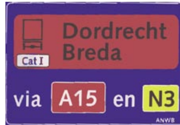
Figure 11: Panel showing alternative route for carriage of dangerous goods
