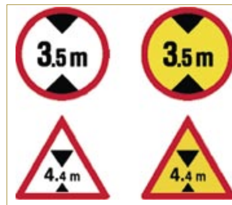
Figure 9: The international sign C6 (above) prohibiting over height vehicles and the sign used in the UK (below)
